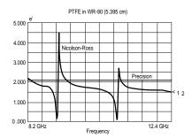
Air gap correction algorithms increase the accuracy of measurements made in a transmission line media.
