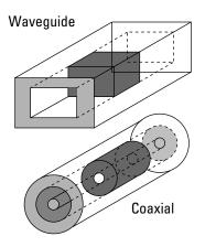
Simple coaxial or waveguide transmission lines hold the samples of material under test.
