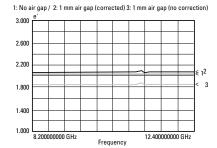
Traditional methods produce spurious data at periodic frequencies. With the HP 85071B you get accurate data at all frequencies.
